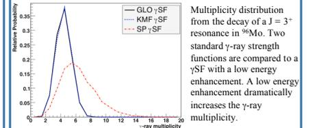
Multiplicity distribution from the decay of a  $J = 3^+$  resonance in  $^{96}\text{Mo}$ . Two standard  $\gamma$ -ray strength functions are compared to a  $\gamma$ SF with a low energy enhancement. A low energy enhancement dramatically increases the  $\gamma$ -ray multiplicity.
