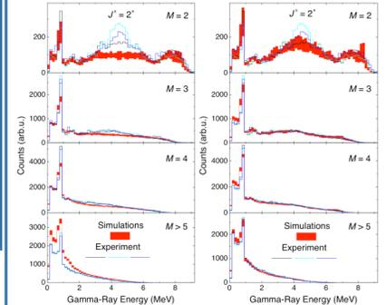
$\gamma$ -ray spectra from the decay of  $J = 2^+$  resonances. The spectra are plotted according to the multiplicity of the  $\gamma$ -ray cascade,  $M$ . The spectra on the left are compared to simulations with a low energy enhancement while the spectra on the right are compared to simulations with an empirical  $\gamma$ SF intermediate between a KMF  $\gamma$ SF and the Oslo  $\gamma$ SF.
